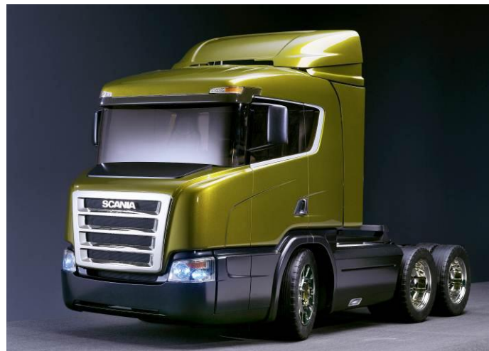
Figure D-31: Scania Crash Zone Concept Truck with extended front end (Scania, 2003)
