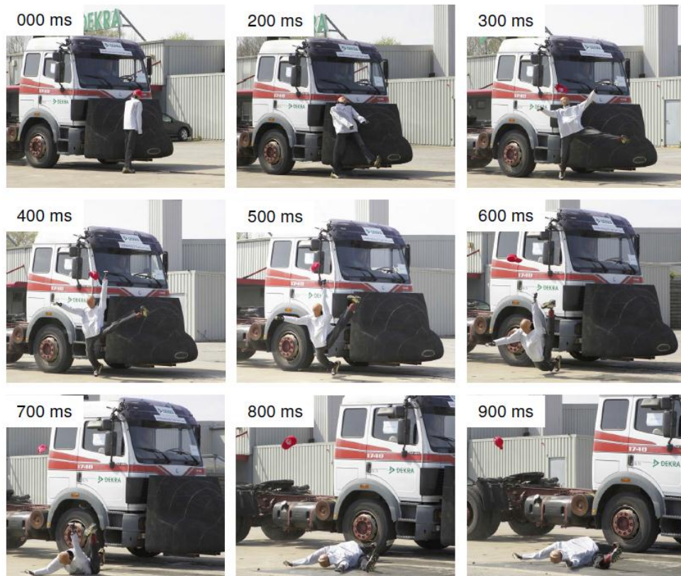
Figure D-27: APROSYS nose cone attached to an HGV front end deflecting a pedestrian dummy to the side in an impact test (Feist and Faßbender, 2008)
