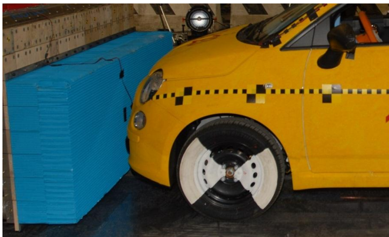
Figure C-9: FWDB test showing deformable element and LCW
