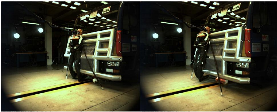
Figure D-26: APROSYS safety bar impacting a standing pedestrian dummy (Feist and Faßbender, 2008)
