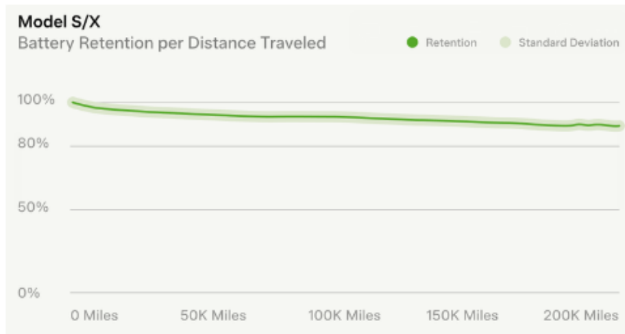
Figure A3.1-4 Tesla Model S/X Battery Retention vs Mileage
